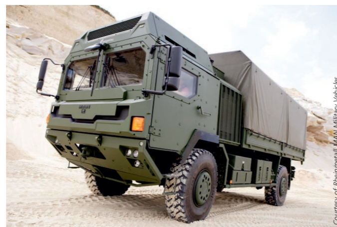
MAN – HX with customized air-conditioning system FSA, integrated into the roof
