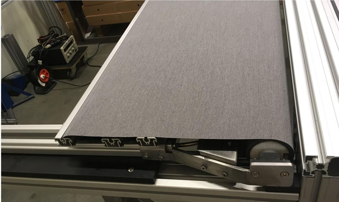
Due to the smart, straight forward design, the retractable Rolling Shade System can be customised in length, width and cross curvature as well as Sunbrella fabric colour options to integrate into any boat design.
