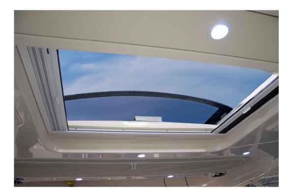
The 40 Series Marine roof is a standard sized and electrically operated roof system that features 8mm tinted safety glass with an attractive design.
